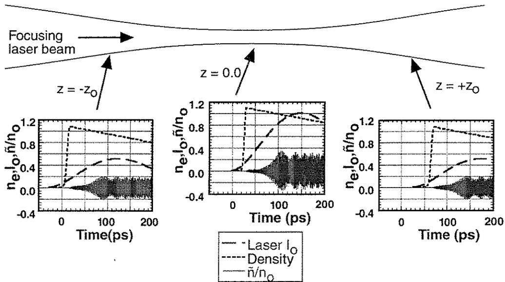
Figure 1.2: 1-D Model to Predict Wave Amplitude vs. Space.
