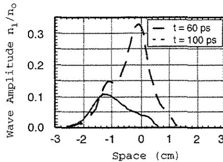
Figure 1.3: Wave Amplitude vs. Space at  $t=60$  and  $t=100$ , based on the 1-D Model.
